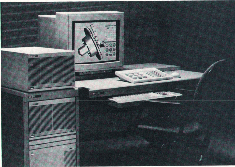
Fig. 1. The HP 9000 Model 825 is a midrange, compact, NMOS VLSI implementation of HP Precision Architecture. It is designed for both single-user workstation and multiuser applications running the HP-UX operating system. The SPU is the middle unit at left.
